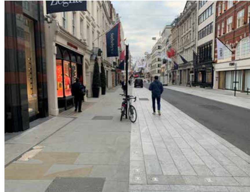
Recessed parking bays within high-quality pavement embody the concept of shared space and provides extra space for pedestrian footways (New Bond Street)
