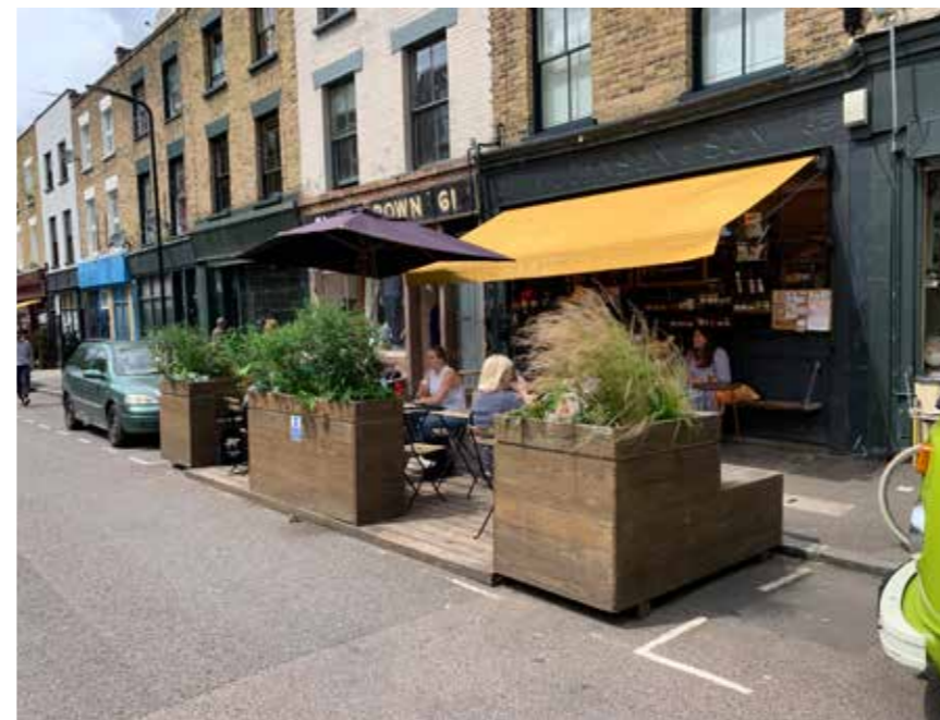
Parklet was built over parking space to create extra floor space for restaurant business (Wilton Way)
