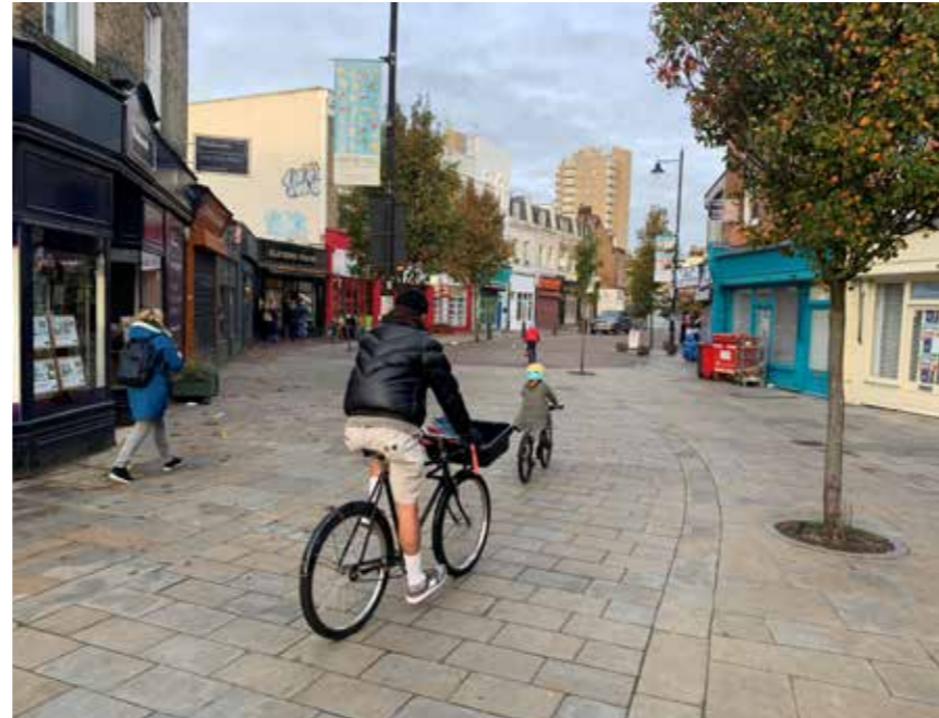
Herne Hill Station - cycle route demarcated with smaller setts
